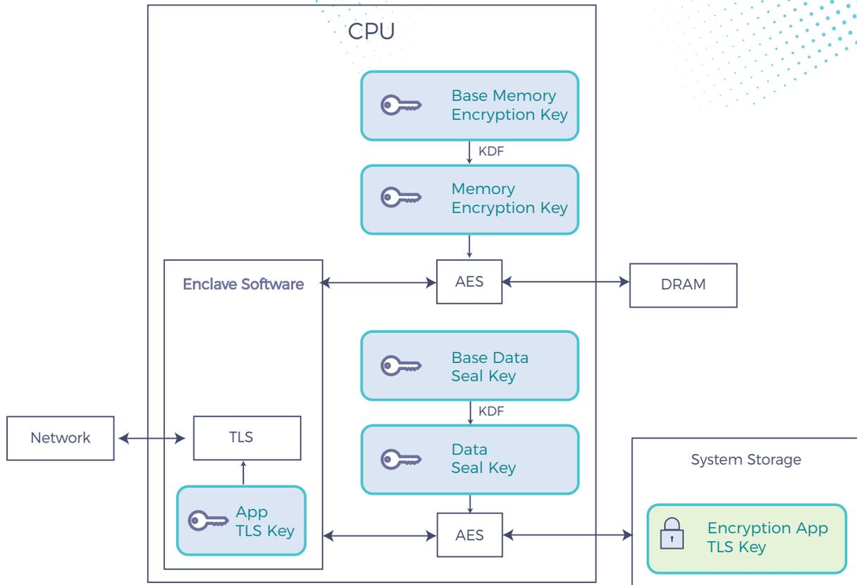
Figure 4: Key hierarchy for storage and network encryption
