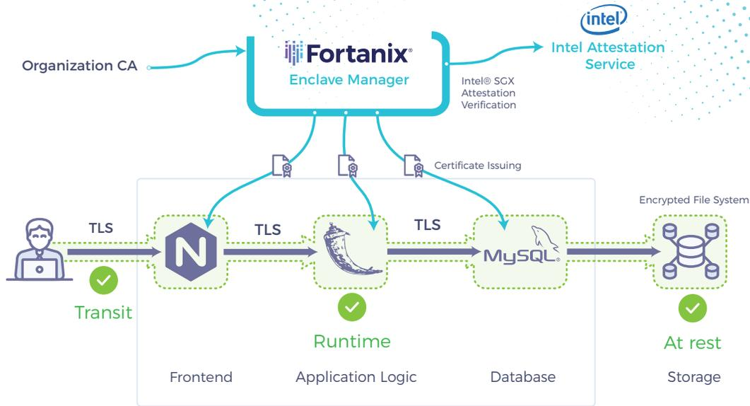
Figure 2: Enterprise 3-tier application secured with Fortanix Runtime Encryption
