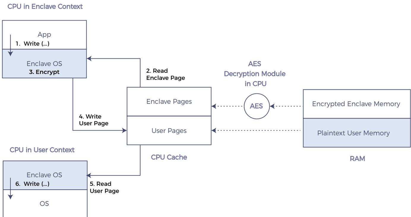
Figure 5: Transparent encryption and integrity protection of memory
